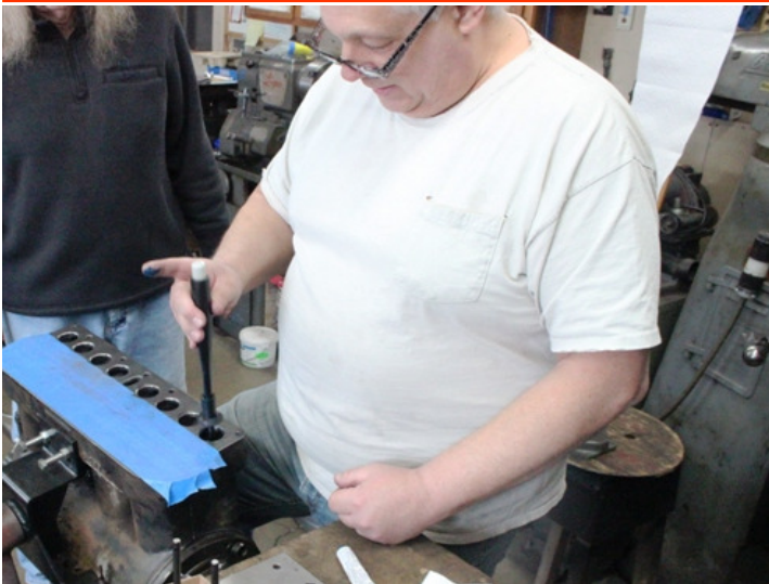
Checking the valve & seat for seal
